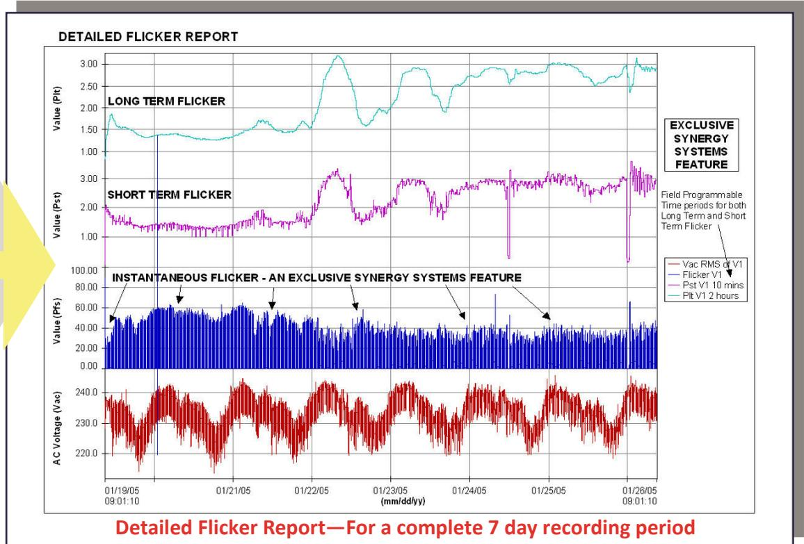
The above Graph is the True RMS value of the Voltage Channel being tested for FLICKER.
