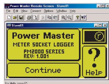
It will not be this screen every time you access the PM2000 – it will be however you left it. The PMScreen application program ONLY provides a screen space and mouse interface. The screen *content* comes from the logger itself, hence if you close PMScreen and re-open it later, the logger screen is likely to be the same as it was when you last looked at it.
